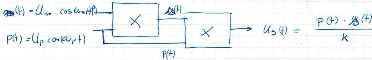
$$u_3(t) = \frac{U_1}{2} \left( \cos((\omega_p + \omega_m)t + \varphi) + \cos((\omega_p - \omega_m)t - \varphi) \right) \cdot \cos(\omega_p t)$$
